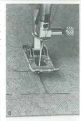
Sewing the buttonhole Place the material under the foot so that the edge of the material lies in front of the presser foot (Fig. 4).
