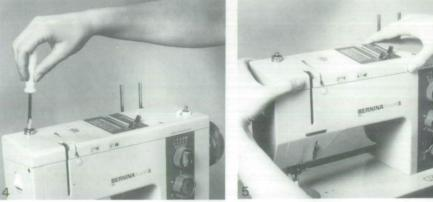
**Dismantle top frame** cover when lubricating Screws 175 and 165 hold the top frame cover secure. Press screws down with screwdriver and turn a half turn right in the clockwise direction (bayonet locking system) (Fig. 4). Top frame cover can then be lifted off (Fig. 5).
