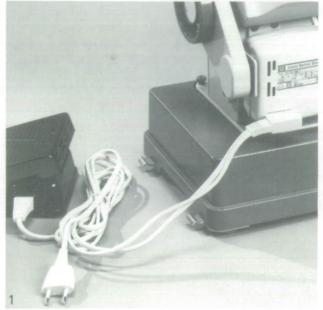
**Connecting mains cable and foot control unit** The terminals on the machine for mains cable and foot control unit can be seen in Fig. 1.
