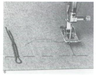
Finally pull the loop of the cord into buttonhole. In knitted fabrics thread ends of cord to rear with large hand sewing needle (Fig. 9) and tie or sew in securely. The cord end can be cut off in woven material.
