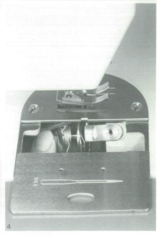
Removing Bobbin Case Open needle plate slider. Turn hand-wheel towards you until the needle is in the uppermost position. Grip bobbin case by the latch with thumb and index finger of the left hand and remove it.
