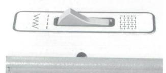
**Darning:** The feed-dog is lowered by switching the changeover switch to the right i.e. to the darning symbol.
