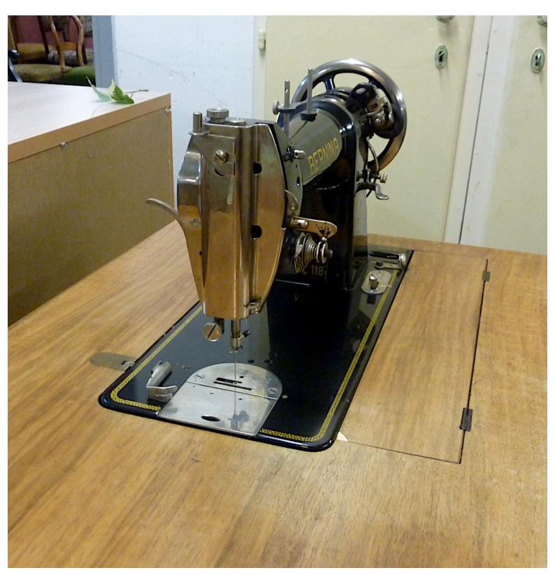
mechanical like the model 105 but with rotary hook like the model Bernina KL 117... and needle type 287 WH
